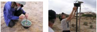
Dust traps created by Marith Reheis of the US Geological Survey. Dust traps T68, T67, T66, T64, T63 and T*6 (no longer extant) are located in Owens Valley (see map)
